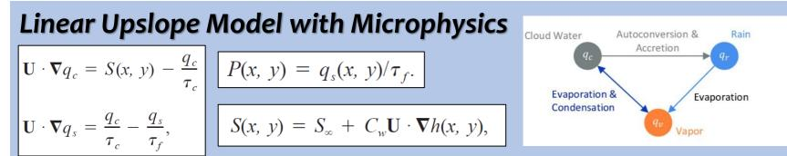
A pair of steady-state advection equations describing the vertically **integrated cloud water** density qc(x, y) and hydrometeor density qs(x, y). where  $\tau c$  is the time constant for conversion from cloud water to hydrometeors (i.e., rain or snow) and  $\tau f$  is the time constant for hydrometeor **fallout**. The model is vertically integrated, we use average values of the time constants, range from **200 to 2000 s**, representative of the whole column.
