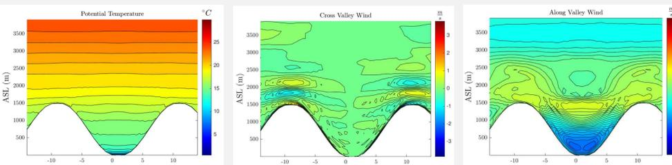
Cross section of potential temperature (left), cross-valley wind (center) and along-valley wind (right) at 03 UTC from the RANS simulation with the BouLac turbulence parameterization and the Noah LSM.
