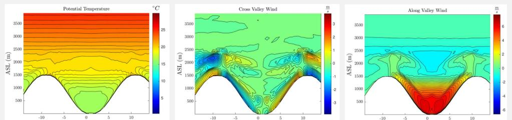
Cross section of potential temperature (left), cross-valley wind (center) and along-valley wind (right) at 15 UTC from the RANS simulation with the BouLac turbulence parameterization and the Noah LSM.
