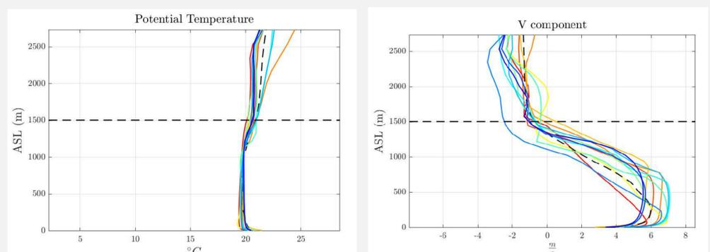
Vertical profiles of potential temperature (left) and along-valley wind (right) at 15 UTC from the RANS simulations and the LES.
