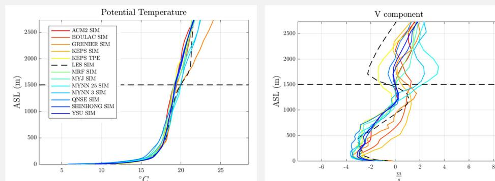
Vertical profiles of potential temperature (left) and along-valley wind (right) at 03 UTC from the RANS simulations and the LES.
