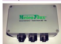
This is the task of (to mention the unit actually used in this work) MeteoFlux® Core V2: a real-time "eddy covariance" system.
