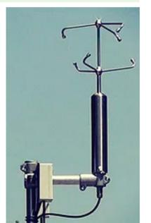
An ultrasonic anemometer is not enough, however: the instrument produces a stream of very high resolution wind and temperature data. The mass of readings is just too much to be of immediate use, and a real-time processor is then indispensable to distill useful data and information from it.
