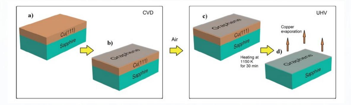
Raman and light transmission characterization of Gr/Al2O3 show enhanced quality by tweaking Cu removal conditions [3]
