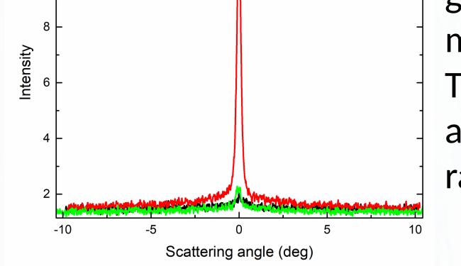
grown by a newly developped method [2]. The film is transparent. The specular He reflection intensity and FWHM indicate flatness and long range crystalline order.
