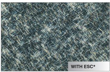
The photos above illustrate silver nanowires sprayed without ESC (top) and with Ultrastatic® ESC (bottom) using the same deposition parameters.
