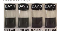
The efficiency of Polarclean for obtaining high-yield and stable dispersions of flakes
