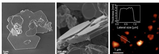
The representative AFM and the corresponding height profile collected along the white line, allow concluding that Polarclean assisted LPE provides flakes with an aspect ratio of ~10<sup>3</sup>.
