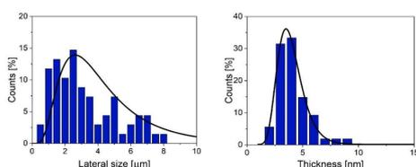
Statistical analysis of lateral size and thickness of WS<sub>2</sub> flakes based on SEM and AFM images demonstrate that lateral size and thickness of the flakes approximately follow log-normal distribution peaked at ~3 μm and ~4 nm respectively.
