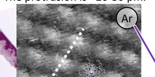
At а protrusion of ~60 pm indicates O<sub>2</sub> adsorption.
