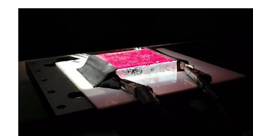
Experimental setups for testing the optical and electrical efficiencies of LSC devices.
